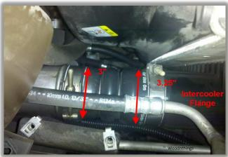
Passenger side intercooler boot (cold side). This is located under the degas bottle. (degas bottle removed)
