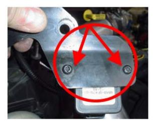
4. The picture to the right shows where the MAP sensor must be mounted on the new bracket from Riffraff Diesel's OCR kit. The bottom picture shows the proper orientation for the sensor so it will fit under the cowl when mounting the new OCR bracket back into position.
