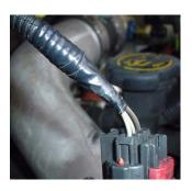
3. Using either the T20 driver or flat tip screwdriver, remove the two screws which hold the MAP sensor to the sensor bracket. Either save or discard the sensor bracket as it will no longer be required.
