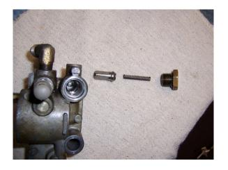
The main FPR seat valve is straight forward - seat, spring and cap in that order. Install the new o-ring on the brass FPR cap (use the **O-ring #8**). Lube the o-ring area with some light oil or motor oil and screw it into the port making sure the spring is center on the pointed spike on the brass plug.
