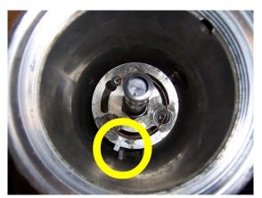
Place the heater element on the stand pipe port with the tab of the element plate **to the left** of the aluminum tab cast into the fuel bowl. These tabs keep the heater element from turning while tightening the stand pipe and causing damage to the electrical wire and connector.
