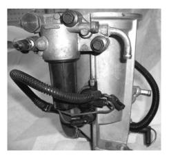
You can now remount the fuel bowl in the engine bay and reconnect the wiring harness and fuel hoses. It will be necessary to connect the hose attached to the bottom of the fuel bowl prior the bolting the bowl to the engine.
