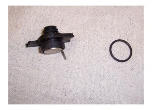
After cleaning the Heater electrical connector, use the **O-ring #4**. Lube the o-ring area with some light oil or motor oil and insert it back into the heater port on the fuel bowl. Rotate the connector so the tall tab interlocks under the tab cast in the fuel bowl.
