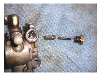
Here is the Fuel Pressure Relief Valve removed from its containing port. There are only three parts to this valve, the seat, spring and brass cap. Set all these parts aside to be cleaned in the parts cleaner tray.
