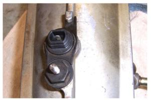
After cleaning the Water In Fuel Sensor, use the **O-ring #6**. Lube the o-ring area with some light oil or motor oil and screw it back into the WIF port below the Heater connector.
