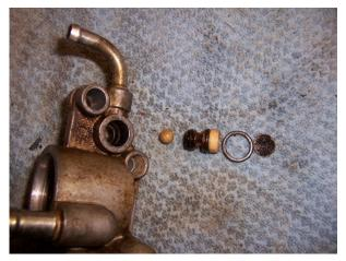
Be very careful removing the bleeder orifice as there is a check ball sitting in the recess below it. This check ball has a lot of bounce and will be difficult to locate if it falls out and decides to leave. In this photo you can see the check ball, bleeder orifice with the two o-rings, the sealing o-ring between the FPR and the fuel bowl body and the screen.
