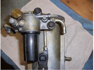
Place the cleaned screen filter into the port opening on the fuel bowl and set the new **O-ring** #5.into the recess.
