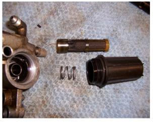
The 1994-1995 models have a screen filter canister that is attached to the FPR. It simply unscrews from the FPR. The screen element slips over the tube that is cast into the FPR and the spring that sits in the bottom of the canister holds it in place. You will want to use a soft bristle brush to thoroughly clean the filter and blow dry with compressed air.
