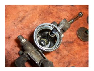
(96-97 Only) There is a plastic snubber that is in the port leading to the Fuel Restriction Sensor that can be removed by gently prying it out with a pick tool. This will open the internal port for additional cleaning.
