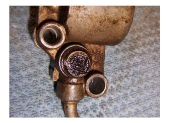
Here is the small screen that is located between the FPR and the fuel bowl. Notice the accumulation of debris on the screen that almost occludes the flow of fuel into the FPR. The screen is sitting on what appears to be a white nylon part that functions as a bleeder orifice for the FPR. There are two o-rings on this white bleeder orifice.
