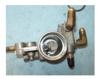
(96-97 Only) When removing the c-clip and plate from the regulator assembly, the filter is exposed. This filter can be removed and washed in solvent until the fluid runs clean.
