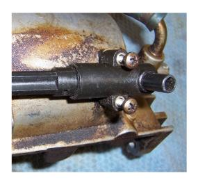
Remove the Fuel Drain Valve: Use a #2 Phillips screwdriver and remove the 2 machine screws that hold the valve to the bowl. The extension handle will separate from the valve once the unit is removed. The keyway is configured so the handle extension will only couple with the valve in one position so there is no need to be concerned with handle orientation. Set the drain valve aside to be cleaned with the other parts.
