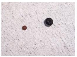
(94-95 ONLY) There is a small check ball and cover located under the upper fuel bowl drain valve port. Carefully remove this cup and ball from the port as you will need to clean the area and the parts may become dislodged during the process of cleaning the fuel bowl. Set these parts aside for cleaning.
