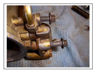
Remove the Fuel Pressure Regulator assembly: Two 10mm head bolts are all that hold the FPR to the fuel bowl. The 94-95 models will have a black plastic canister hanging from the FPR that contains a screen filter within it. The 96-97 models will have a hard line fitting connected to a plate under the FPR. When separating the FPR from the bowl, there is a small screen that may try to fall out from between the two bodies. Watch for this screen so you will not loose it.
