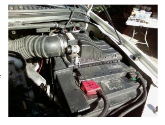
Leaving these protrusions in place helps prevent filter movement.
